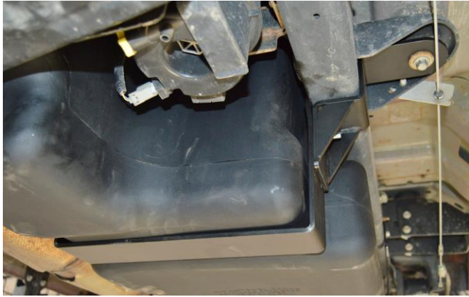
(Fig. 11) Completed front support installation tank.
