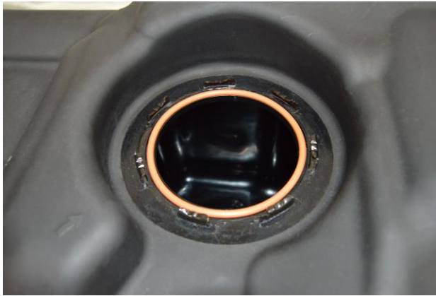
(Fig. 3) O-Ring gasket shown installed correctly.
