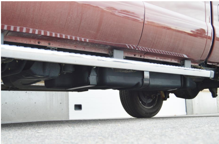
(Fig. 11) Completed front support installation tank.
